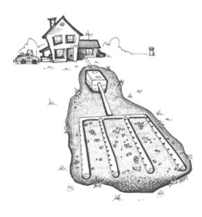
If your home is not on a municipal sewer or community septic system, your wastewater probably goes into an on-site sewage disposal system, commonly called a septic system. A septic system is designed to collect, treat and dispose of wastewater on site so that it can percolate into the ground without contaminating ground or surface waters. In Connecticut, nearly 40% of homes use some form of on-site sewage disposal system to treat and dispose of household wastewater.
