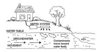
The Septic Tank separates solids from liquids before sending wastewater to the leach field. A layer of sludge settles at the bottom and a layer of scum forms at the top, so only the clearest wastewater goes into the ground. Keeping solids in the tank and out of the leach field is the best way to prolong system life. That means the tank needs to be cleaned or pumped out periodically.
