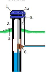
Note: Not all drilled wells are equipped with a pitless adaptor (6.) and a submersible pump. Some well pumps are located inside the home and use suction to draw water from the well.
