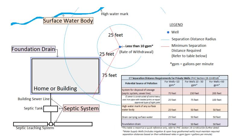
General **well construction standards for private wells** can be found in both the Connecticut PHC and the Connecticut Department of Consumer Protection Well Drilling Code.
